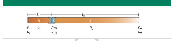
Figure 2: Retention gap and analytical column ensemble. A = retention gap, B = zero dead volume connection, and C = analytical column.
