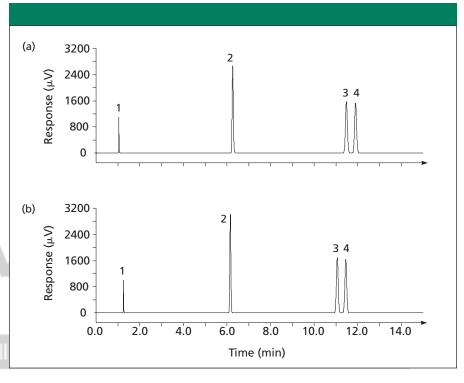
**Figure 1:** Effect of a retention gap on retention and peak shape. (a) 25 m  $\times$  0.25 mm, 0.25- $\mu$ m  $d_{\rm f}$  column, 17.75 psig inlet pressure and (b) same column as (a) with a 5 m  $\times$  0.25 mm uncoated retention gap added to the beginning, 21.6 psig inlet pressure. Conditions for (a) and (b): helium carrier gas, 40 cm/s, 100 °C. Peak profiles calculated from theoretical H values assuming 83% coating efficiency.
